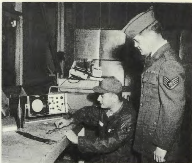
The same type of signal used to check wing spars revealed dangerous crack in the rotary mower blade.
