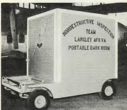
Portable darkroom permits on-the-spot X-ray film processing.
